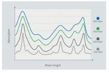
The graph shows how the absorption peaks varies at different pressures (100, 200, 400, and 800 mbar). Lower pressure increases peak sharpness, making the absorption ranges more distinct and reducing interference between different measuring components, resulting in more precise measurements.
