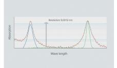
The graph shows the absorption of two gases (blue and green curves). Each gas absorbs specific wavelengths, creating a unique spectrum like a fingerprint. By analyzing the absorption (black line with red dots), the presence and concentration of gases can be accurately detected.
