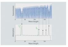
The transmission spectrum (blue graph) shows wavelength changes during measurement, which reveal the absorption spectrum (black graph). Each gas component absorbs specific wavelengths, creating unique peaks in the absorption spectrum.
