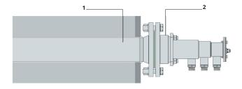
Water cooled: Flange DN80 PN10 with protection tube (1)
